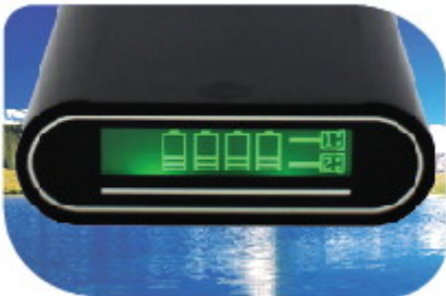
Display showing battery status, charging port, charging current
